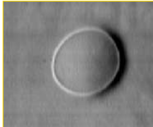
Grayscale image of a bonding gap
