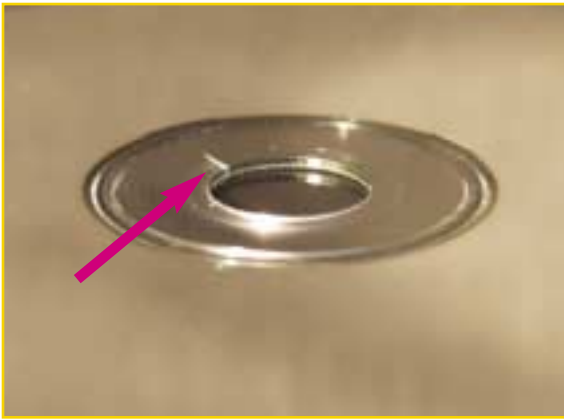
Disc with crack
