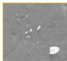
Missing coating (pinholes)
