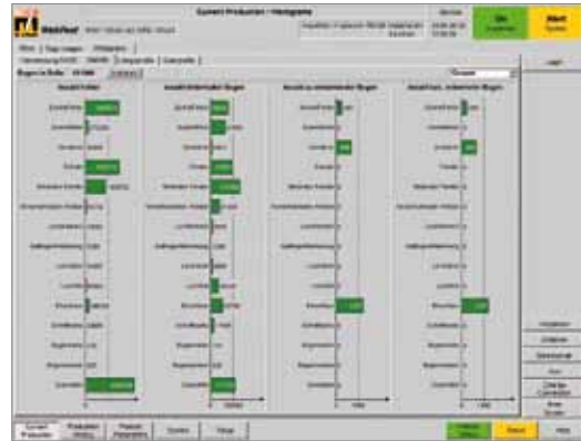
Production Statistics show e.g. number of produced sheets, count of all kinds of defects, as well as counts and reason for rejected sheets.
