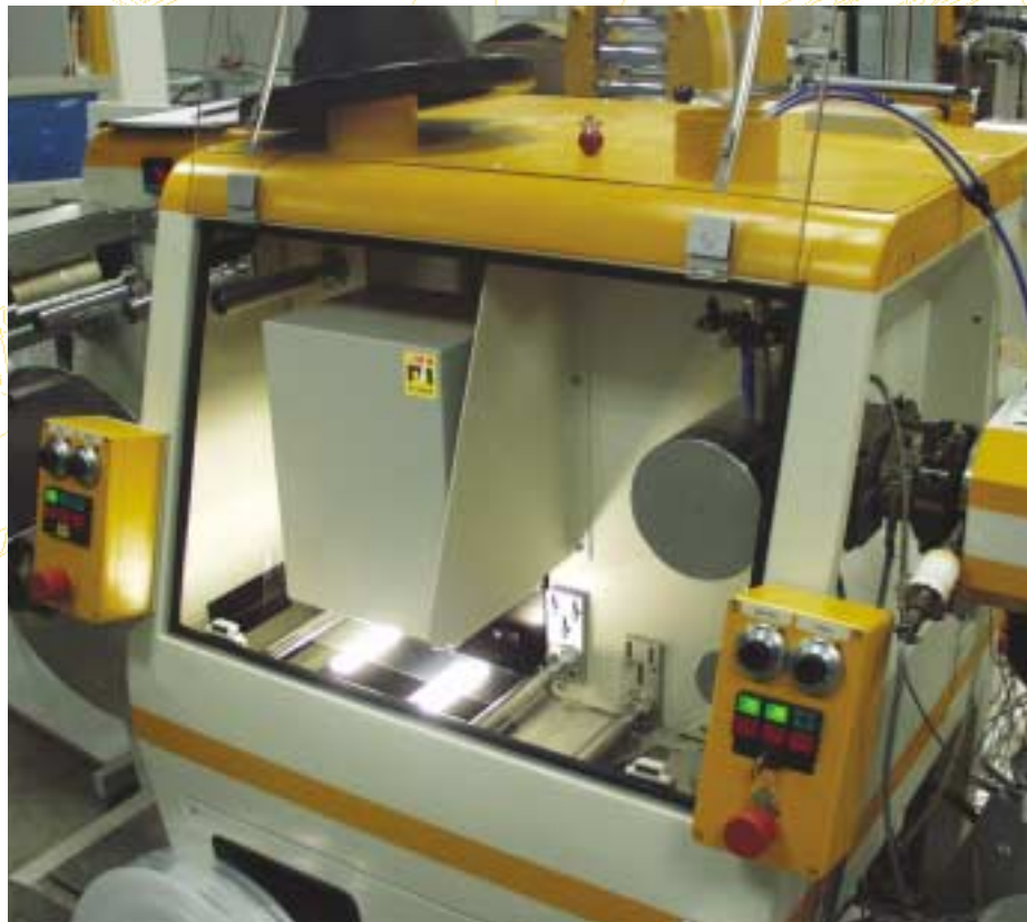
Dr. Schenk Inspection System WebFeat for Plastic Film
