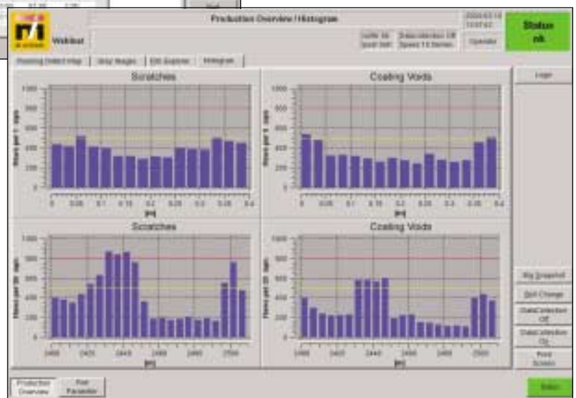
Figure 13: Defect-Histograms as Transverse- and MD-Profile
