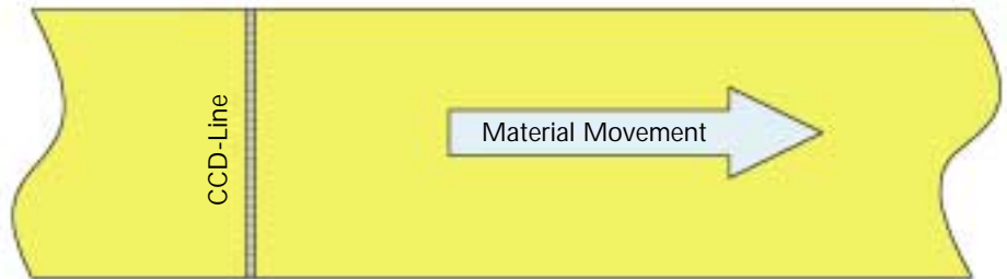
Figure 2: Scanning Principle of Web Inspection
