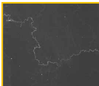
Crazing defect in Low-E coating detected by GlassInspect
