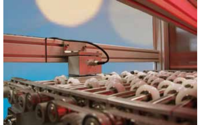
An optional sensor measures the resistivity of the TCO layer on the glass substrate
