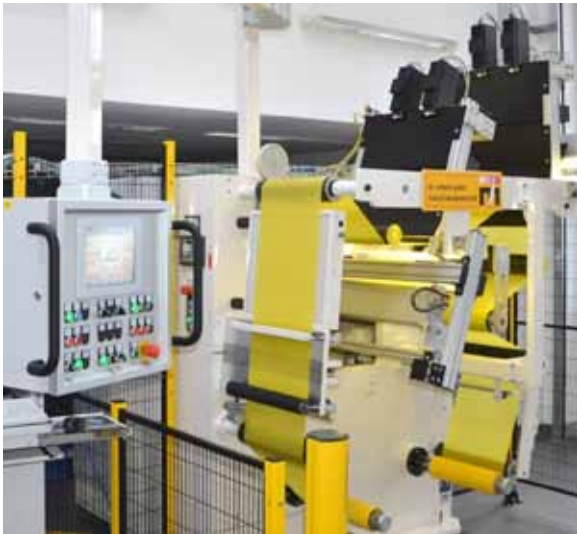
Dr. Schenk inspection system at a rewinder
