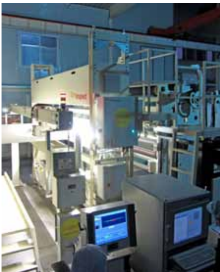
Dr. Schenk inline inspection for nonwoven materials
