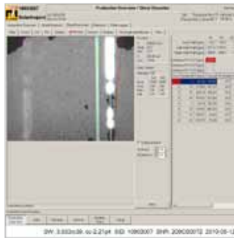
Screen shots of scribe defects: Discontinuities in scribes will result in short circuits
