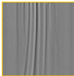
Gel (Top) and Wrinkle (Bottom) defects, displayed in different optical channels
