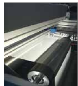
AOI of transparent BOPET film
