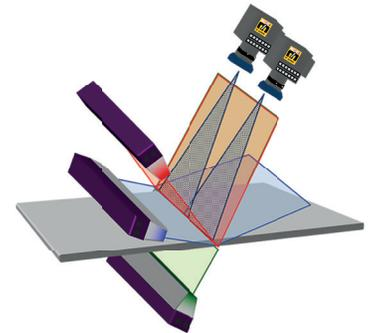
*Dr. Schenk MIDA configuration for battery foil inspection*
