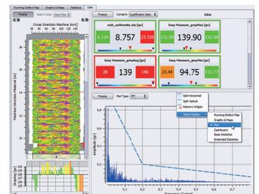
*Integrated Fast Fourier Transformation helps identify interfering periods and frequencies*
