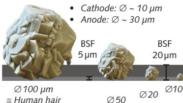
Scale representation of separator film thickness (BSF) cp. with human hair and different sized particles on lithium ion battery electrode coatings
