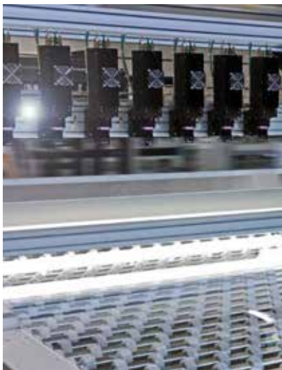
Inline ParticleInspect Solution integrated in Production Line
