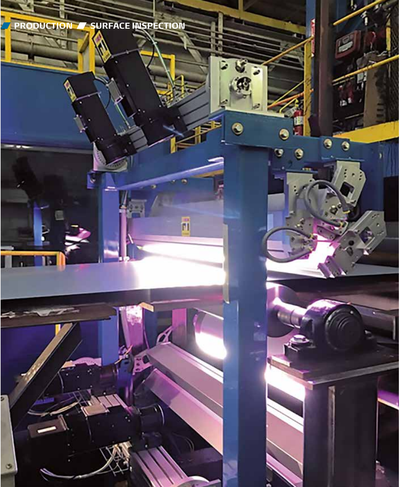
Figure 1: Camera-based surface inspection system with corresponding LED lighting technology on a galvanising line.
