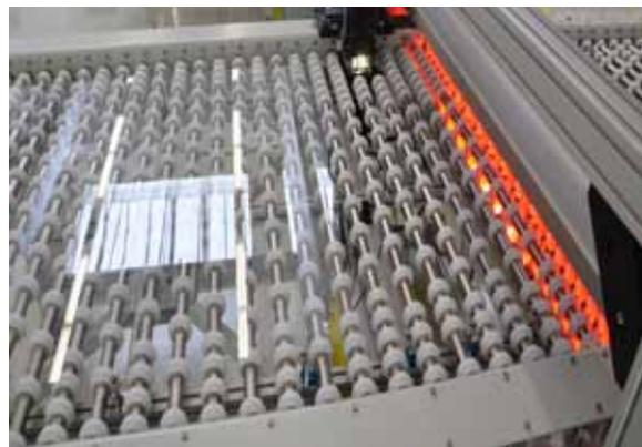
Roller conveyor handling for sheet glass
