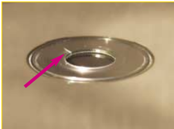
Disc with crack
